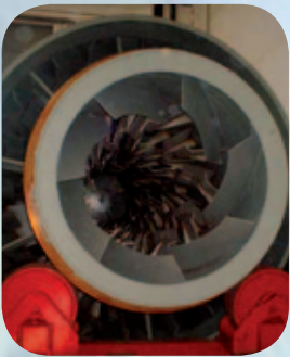
Internal view of the drying chamber
